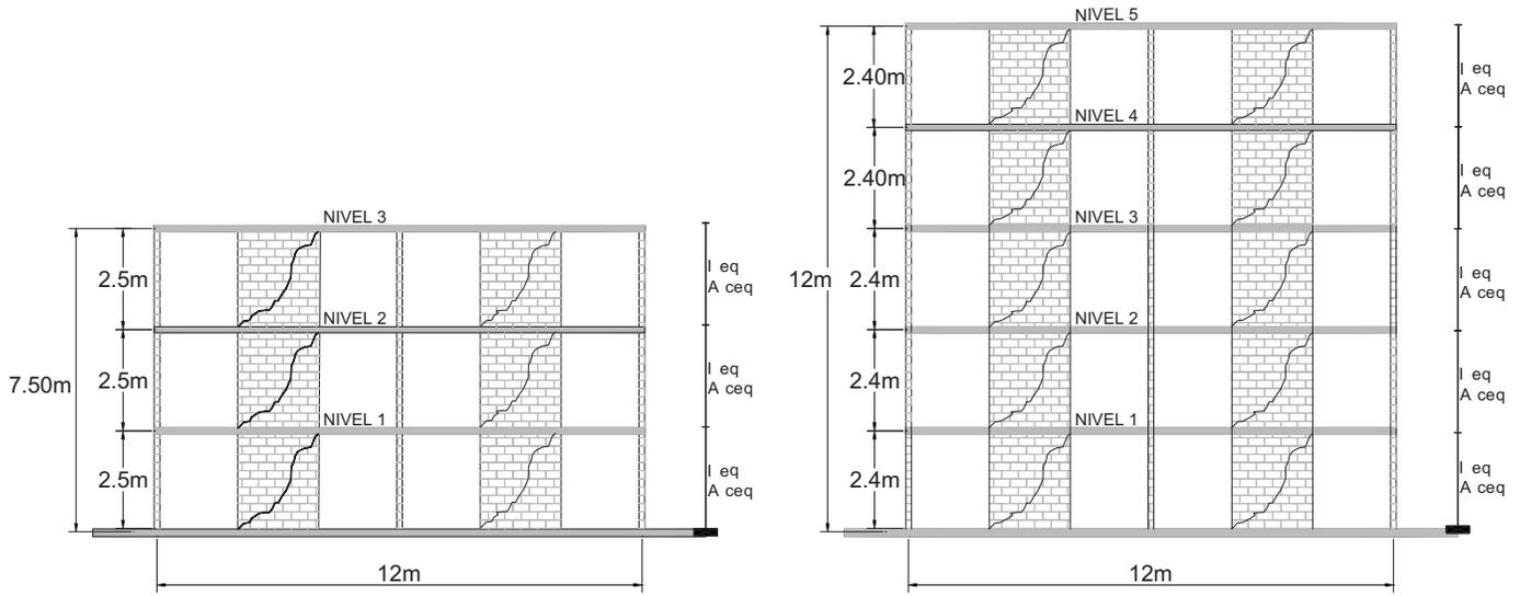
Fig. 11. Elevation of walls running in the horizontal direction for total cracked response
