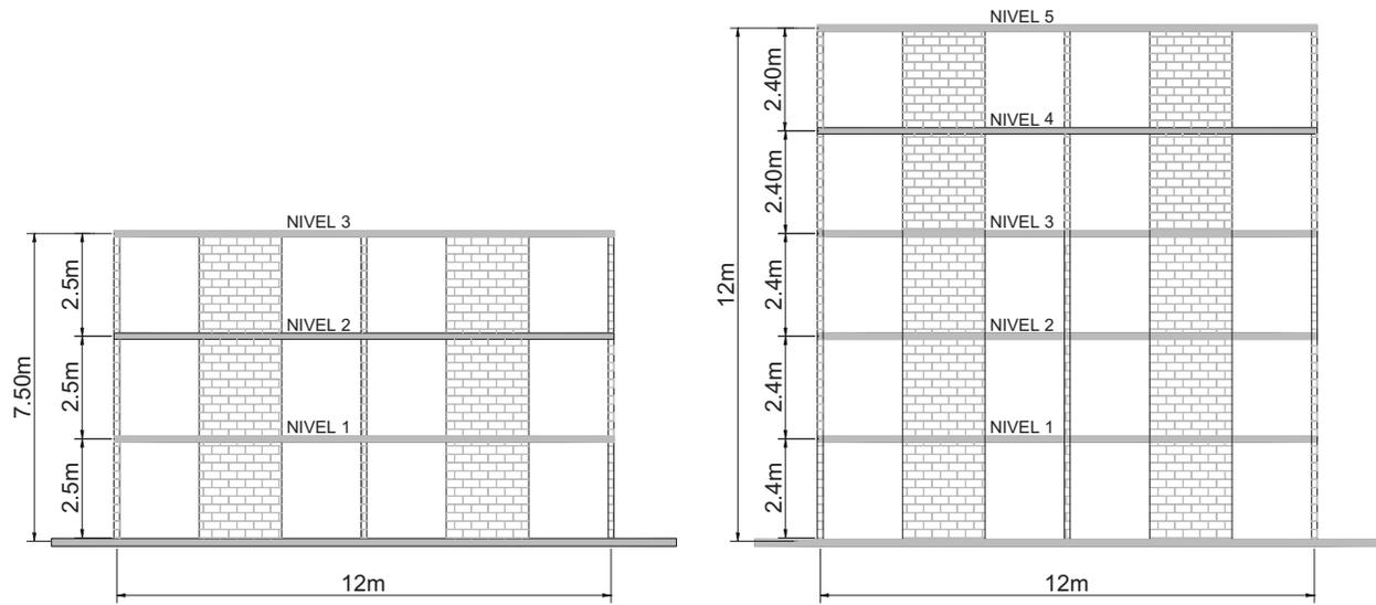
Fig. 9. Elevation of walls running in the horizontal direction for elastic response
