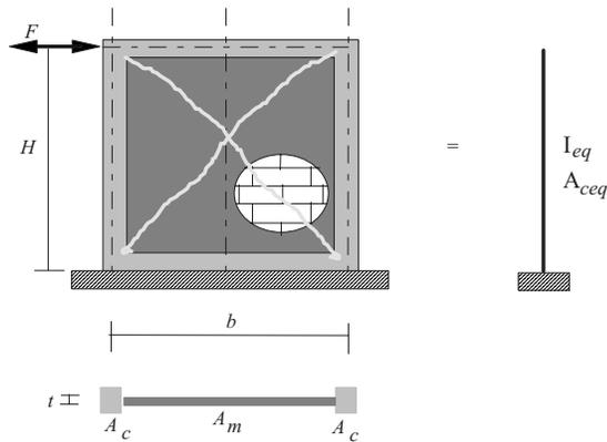
**Fig. 7.** Equivalent cracked wide column analogy proposed by Bazán and Meli
