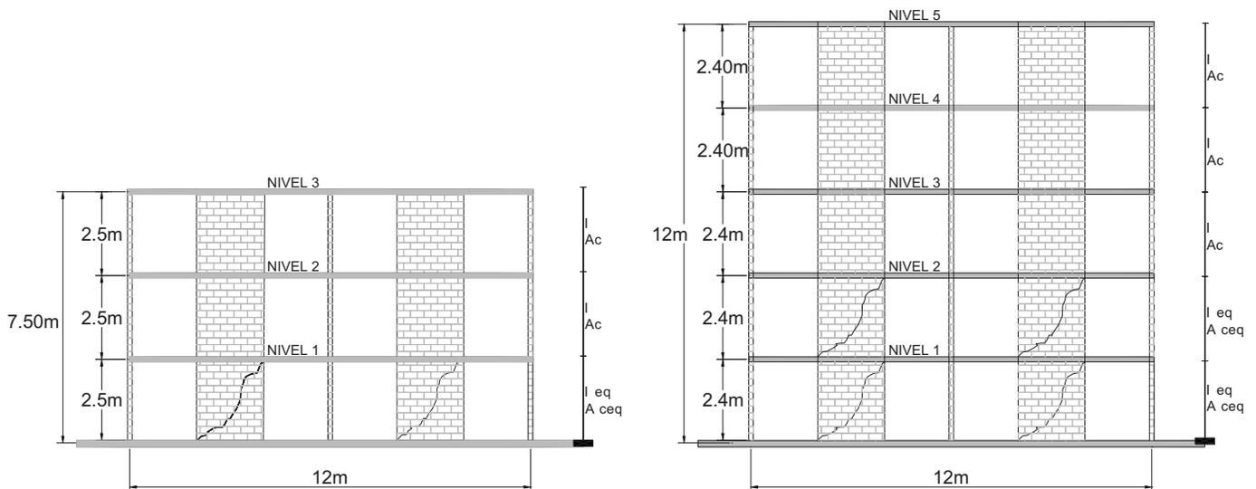
Fig. 10. Elevation of walls running in the horizontal direction for partially cracked response
