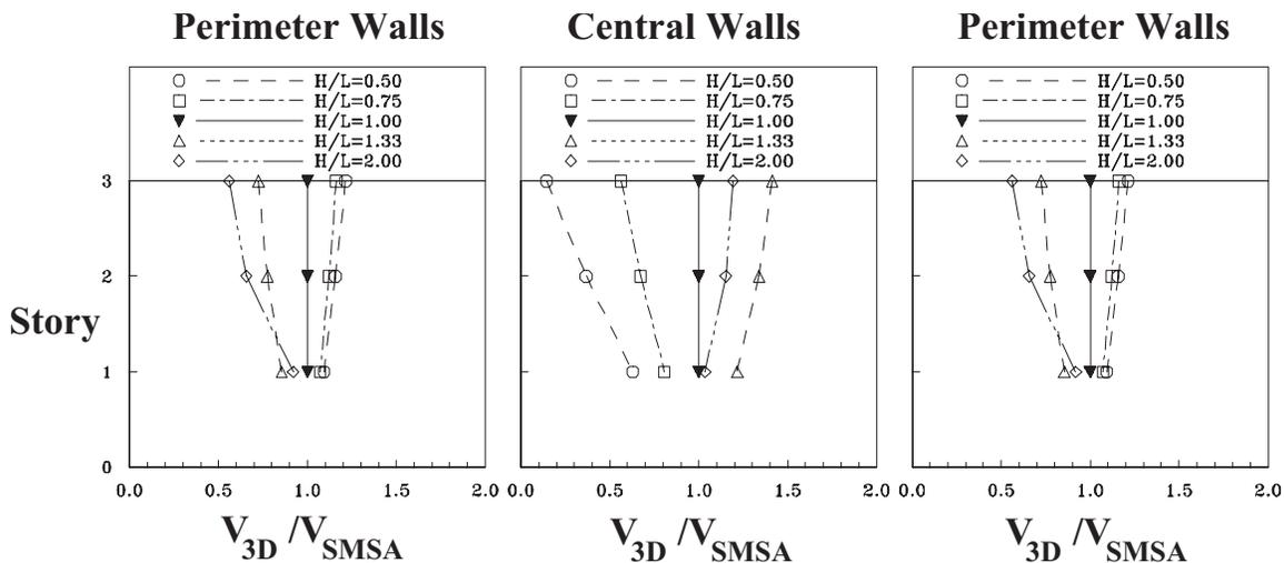
Fig. 6.  $V_{3D}/V_{SMSA}$  ratio for symmetric shear-wall buildings studied by Tena-Colunga and Pérez-Osornio (2001) when subjected to unidirectional lateral load forces
