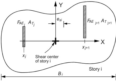
**Fig. 1.** Definition of static eccentricity for the SMSA of Mexican Codes (NTCM-2004 2004)
