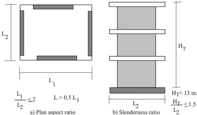
**Fig. 2.** Plan and slenderness requirements for the SMSA
