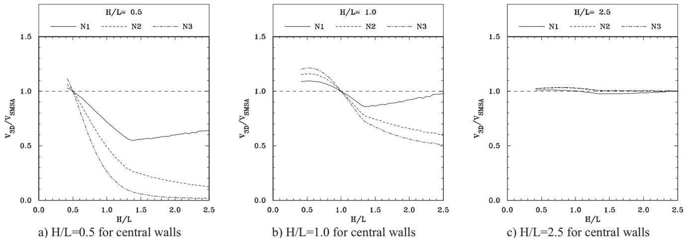
Fig. 12.  $V_{3D}/V_{SMSA}$  ratios for symmetric shear-wall buildings for elastic behavior using current  $F_{AE}$  for the SMSA when subjected to unidirectional static lateral loads
