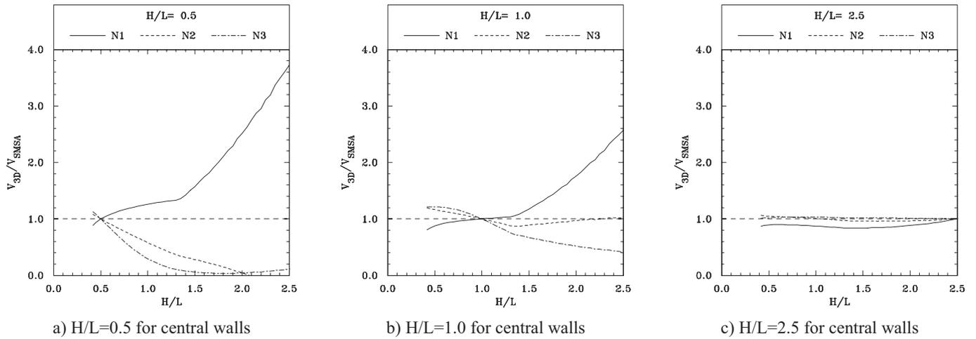
**Fig. 13.**  $V_{3D}/V_{SMSA}$  ratios for symmetric shear-wall buildings for partially cracked response using current  $F_{AE}$  for the SMSA when subjected to unidirectional static lateral loads
