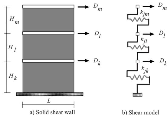
**Fig. 4.** Shear-wall modeling assumption related to the SMSA
