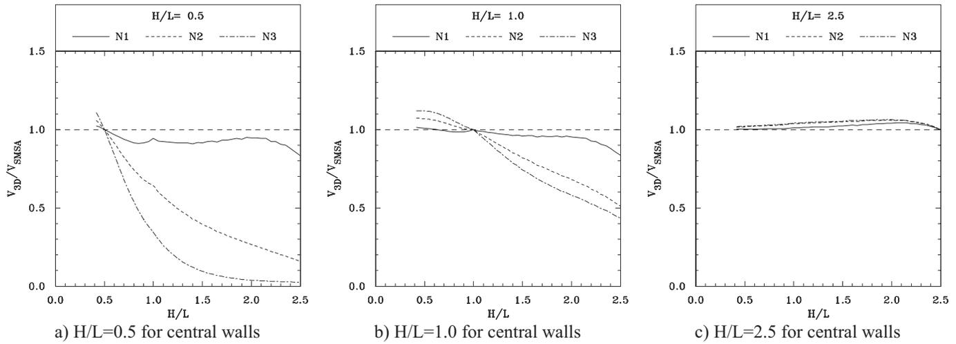
**Fig. 15.**  $V_{3D}/V_{SMSA}$  ratios for symmetric shear-wall buildings for elastic behavior using proposed  $F_{AE}$  for the SMSA when subjected to unidirectional static lateral loads
