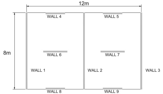
**Fig. 8.** Typical symmetric plan for the bearing wall building models
