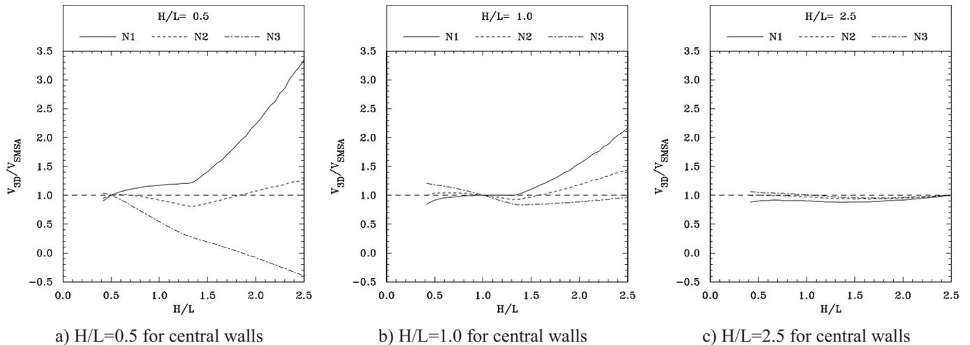
**Fig. 14.**  $V_{3D}/V_{SMSA}$  ratios for symmetric shear-wall buildings for total cracked response using current  $F_{AE}$  for the SMSA when subjected to unidirectional static lateral loads
