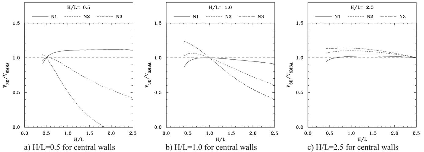
**Fig. 17.**  $V_{3D}/V_{SMSA}$  ratios for symmetric shear-wall buildings for totally cracked response using proposed  $F_{AETA}$  for the SMSA when subjected to unidirectional static lateral loads
