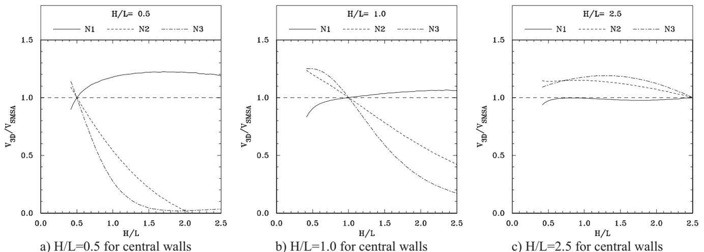
**Fig. 16.**  $V_{3D}/V_{SMSA}$  ratios for symmetric shear-wall buildings for partially cracked response using proposed  $F_{AEPA}$  for the SMSA when subjected to unidirectional static lateral loads
