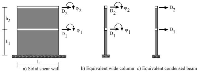
Fig. 5. Flexural wall modeling
