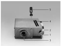
Fig. 30 Mirror housing and illumination telescope 1 Lever for mirror switching, 2 Lateral lamphousing mount with fixing screw, 3 Back lamphousing mount with Allen screw, 4 Illumination telescope for gas discharge lamps
