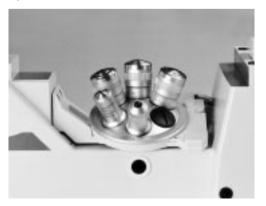
If any positions remain unoccupied, close them with a screw cover to prevent dust penetrating the microscope optics.
