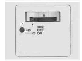
Fig. 69b Bertrand lens engaged (Leica DM IRB)
