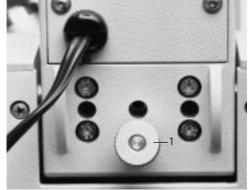
Insert the light rings for Phaco (identified by the code numbers 0, 1, 2, 3 and the intercept distance S of the corresponding condenser top, e. g. 2 S1) and the DF diaphragm (identified by D for darkfield and the intercept distance S of the corresponding condenser top, e.g. D S1, see table  $\rightarrow$  p. 129) in the slots of the disc as follows:
